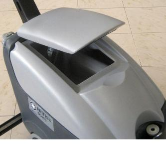
18. Park the machine with the recovery tank cover open
