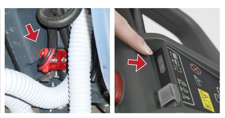
**1** Check if the power cable is correctly **2** Check if the battery is charged. connected.
