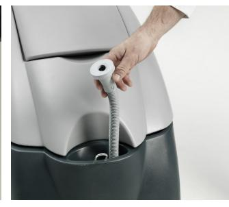
1 Disconnect the battery charger cable 2. Fill the tank with a solution suitable for the work to be performed. Always follow the dilution instructions on the label of the chemical product used to prepare the solution. Its temperature must not exceed 40°C.
