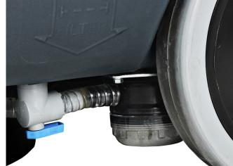
12. Clean the filter by: Remove the transparent cover and the gasket
