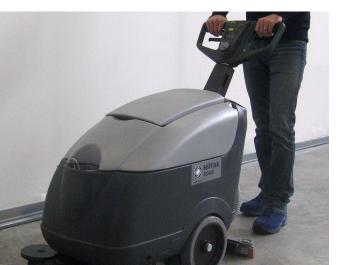
6. Press the handle switch to engage the brush and run the machine
