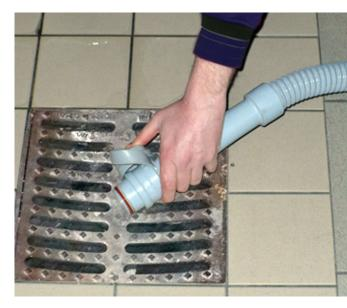
10. At the end of the work. Empty the recovery tank with the hose. Then empty the solution tank with the trasparent hose
