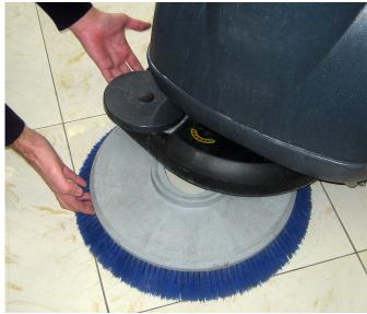
4. Place the brush or the pad-holder under the deck. Use the appropriate brush to clean the floor.
