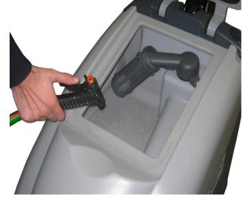
11. Wash with clean water the recovery tank and the vacuum grid
