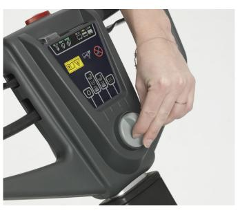
5. Switch on the brush and vac motors to activate the machine
